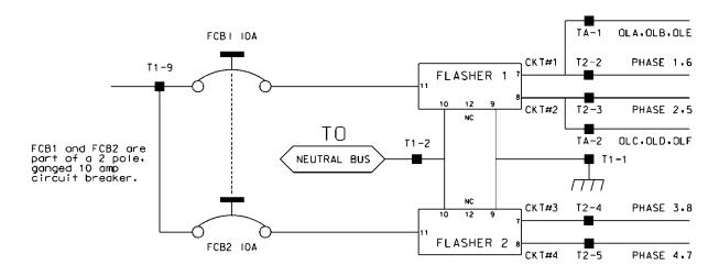
breaker manufacturer to provide gang tripping operation.
